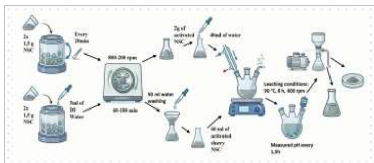
Figure 1. Schematic diagram of dry and wet mechanical activation procedures and subsequent leaching setup.
