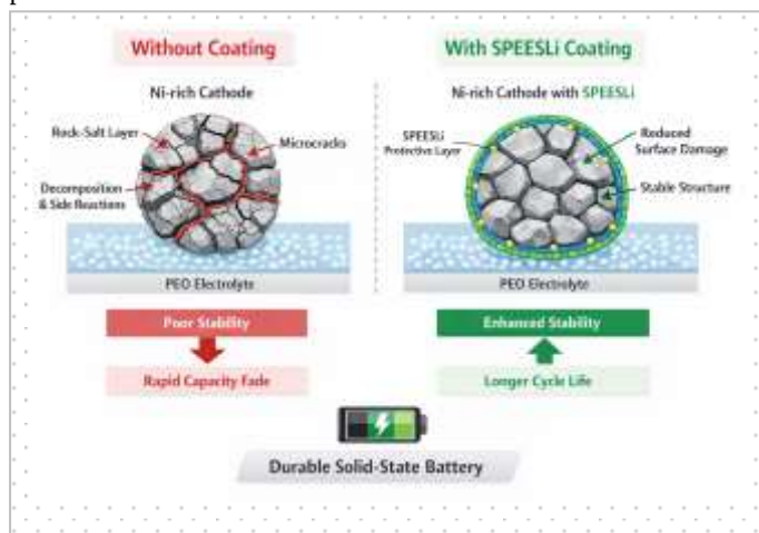
Figure 1. Schematics showing effects of SPEESLi interphase
