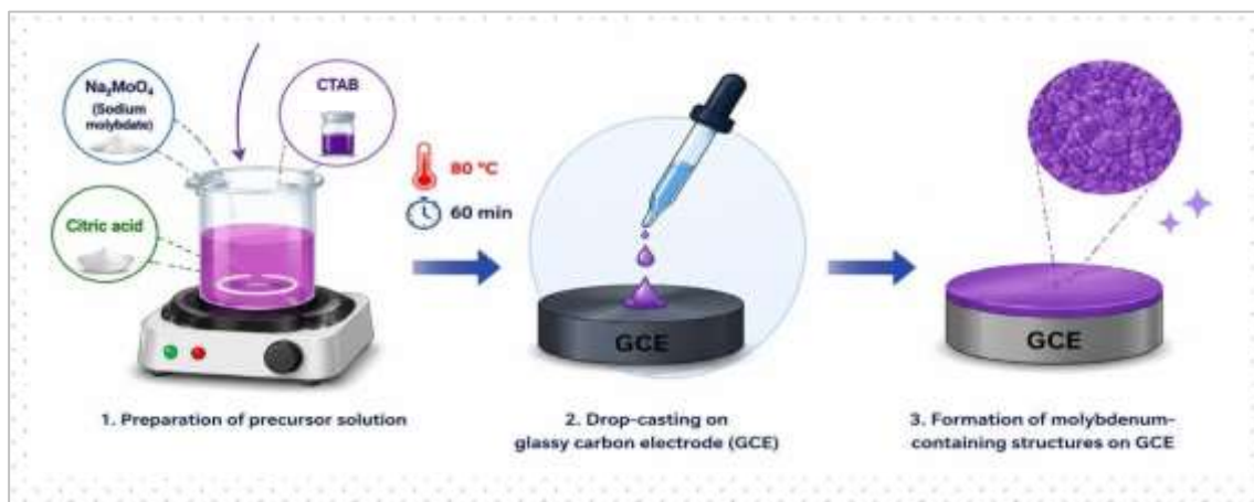
Figure 1. Schematic illustration of the formation of molybdenum-containing structures on the surface of a glassy carbon electrode.
