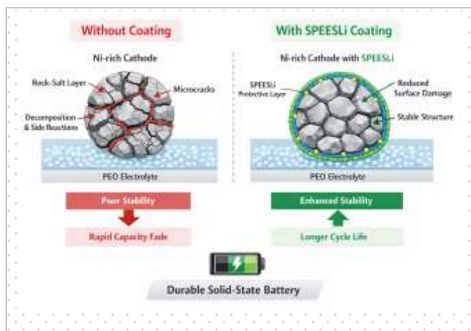
Figure 1. Schematics showing effects of SPEESLi interphase
