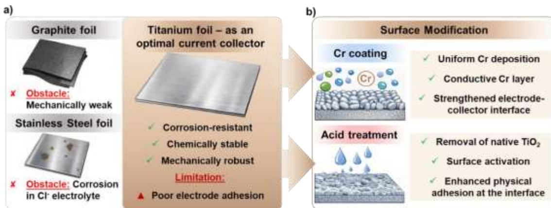
Figure 1. (a) Schematic comparison of candidate current collectors and (b) surface modification strategies for AZLIBs.
