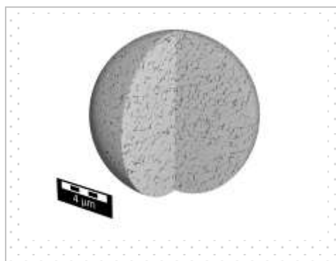
Figure 1. AI generated NMC microstructure for 3D characterization
